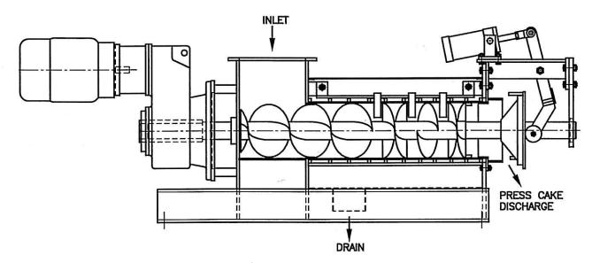
The Model KP Screw Presses are machines in which a screw of progressively reducing pitch rotates inside a cylindrical perforated screen. Material entering the hopper is subjected to gradually increasing pressure as it moves toward the exit end of the press, forcing the liquid phase to extrude through the screen. Dewatering of manure has proven successful over a wide range of applications: scrape, flush, digester, paunch; cow, hog, horse; mixed beddings. Final pressing is controlled
