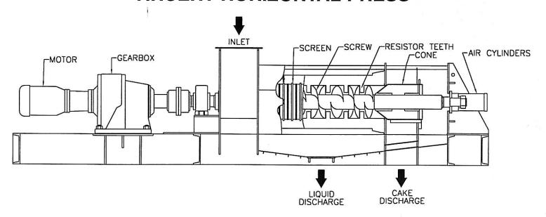
The Vincent Screw Press has proven successful in both virgin fiber and recycle mills. It has a graduated pitch and interrupted flight screw. Final pressing is controlled by a pneumatically actuated cone that adjusts solids content of the press cake. Profile bar
