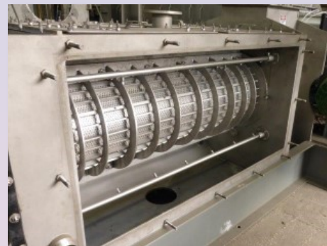
VT Features Include Honey Comb Side Panels, Fitted EPDM Gaskets, and Optional CIP Spray System
