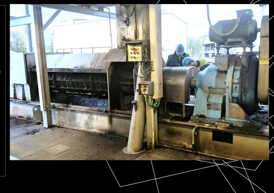
Cover the liquid drain under the screens to prevent lost hardware.
