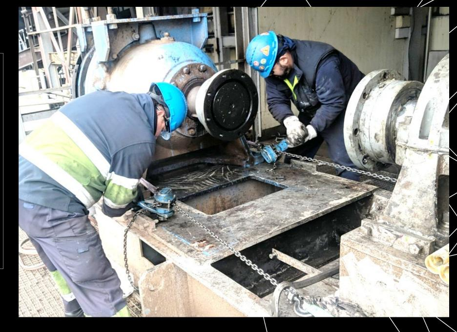
Next, center the discharge end of the screw shaft with the ID of the C-Plate. The tailstock will then be aligned with the screw shaft.
