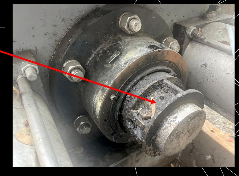
Remove the tailstock/thrust plate assembly (with the air cylinders and thrust bearing still attached).
