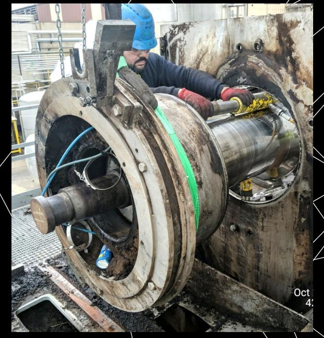
**Remove the** screw from the discharge end of the press, supporting the screw from above as it goes through the vertical plates.
