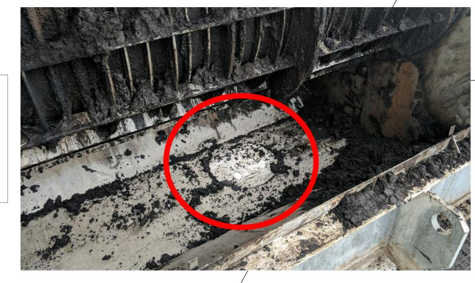
If these angles (used to support screen covers) are on your press, remove them for easier screen removal.
