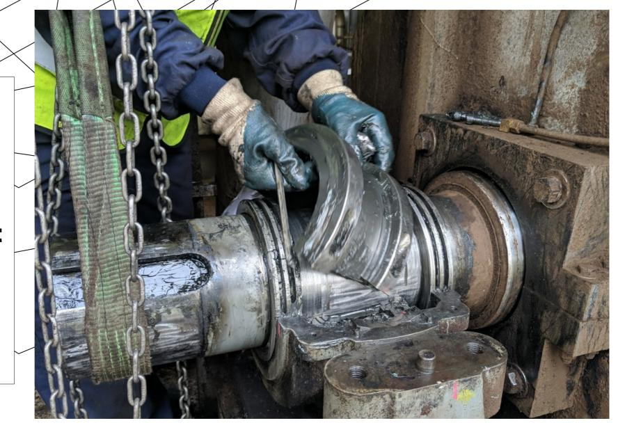
Loosen and remove the four bolts on the seal assembly.
