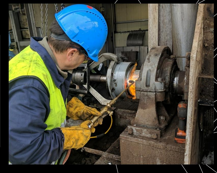
**Remove the pillow block** bearing. (This press had a split **PB bearing.)** If it is a standard bearing (not split), pull it off the shaft.
