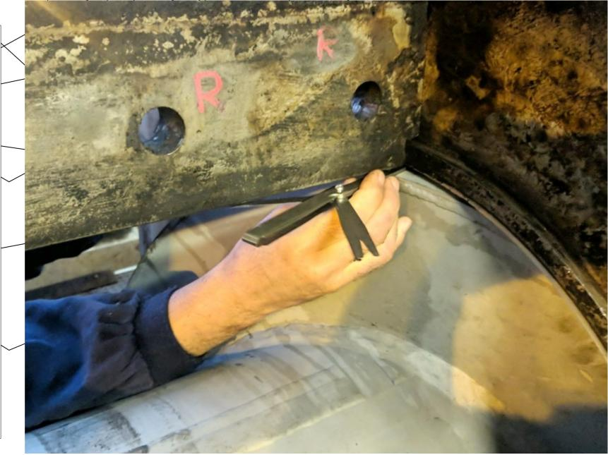
With the screw in place and centered, install the gearbox and align it to the screw. Not the other way around!
