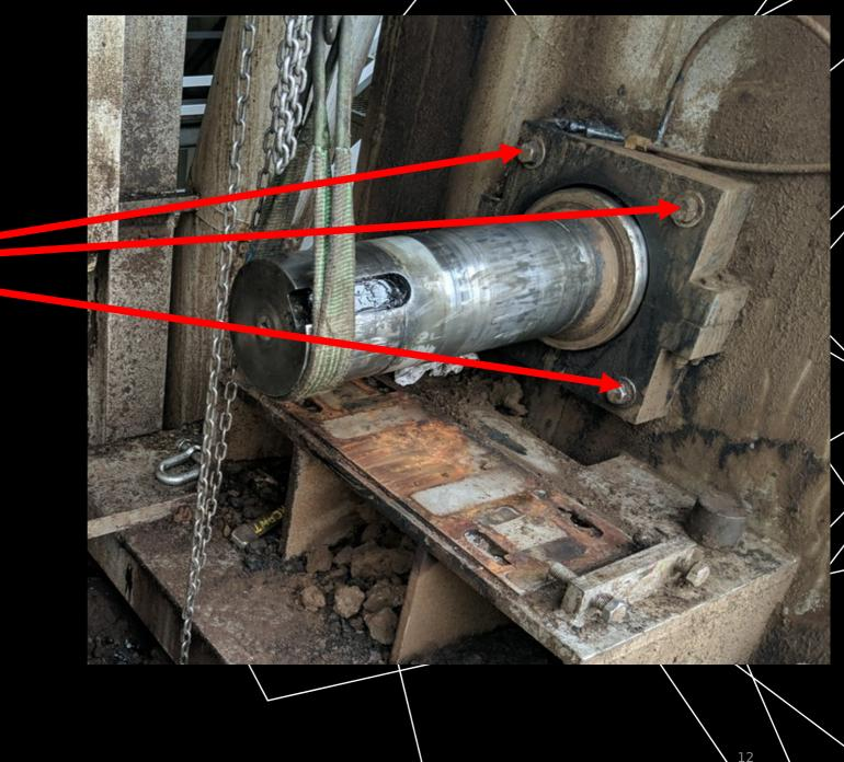
At the discharge end, disconnect the air cylinders.
