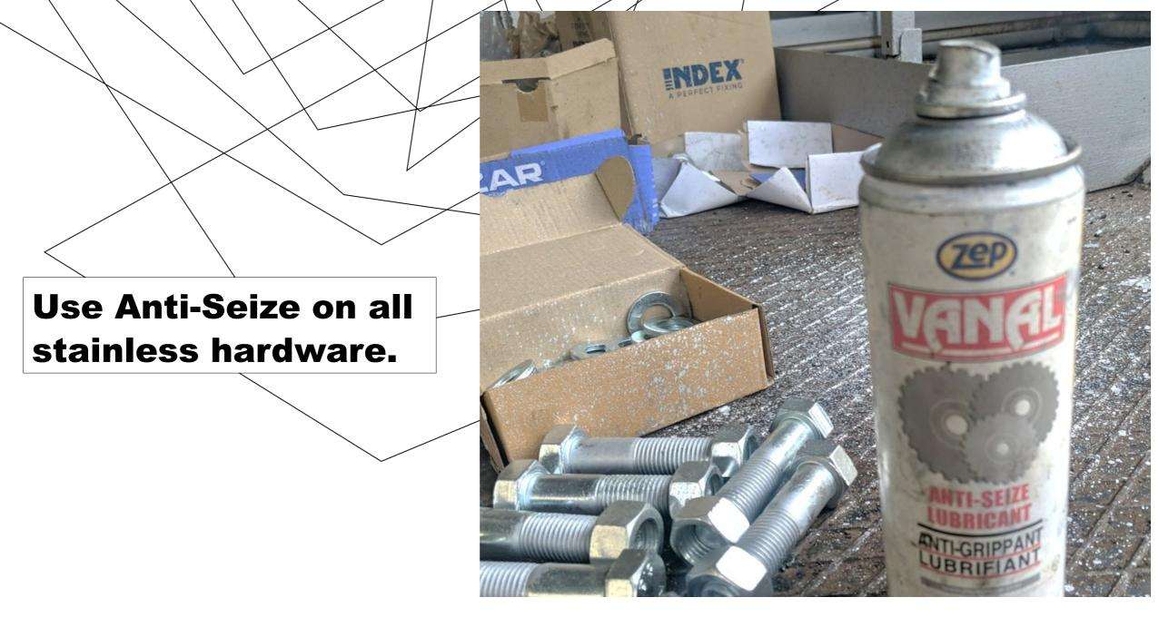
Follow the recommended torque specs for the size/pitch of grade 18-8/304 stainless bolts (Vincent's std. fitment) used on the screens and resistor bars.
