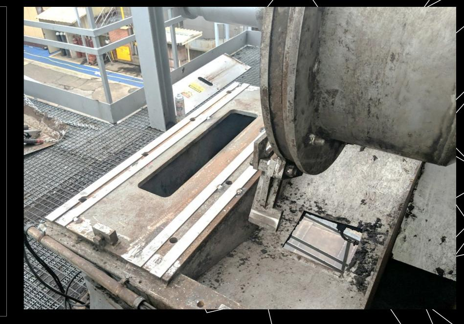
To reinstall the screens, bolt on only one side at a time and measure the gap between it and the screw.
