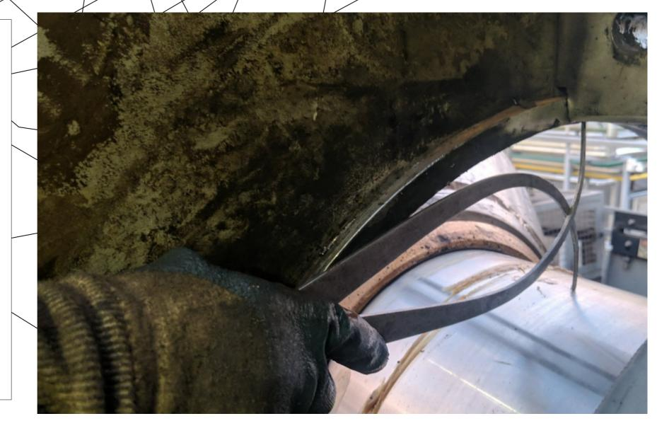
**Reinstall the** discharge cone, tailstock, and air lines. The tailstock should be shimmed to align it with the screw shaft. Again, not the other way around!
