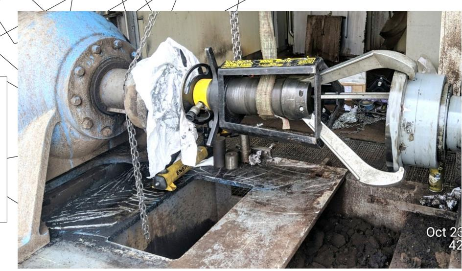
Heat the hub evenly to 300° -500°F (150° -260°C) with a rosebud torch while applying pressure till the hub clears the shaft.
