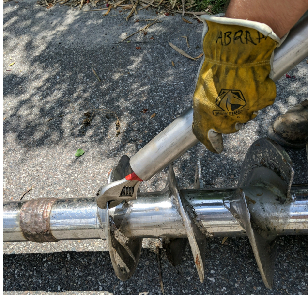
BENDING FLIGHT BACK INTO POSITION
