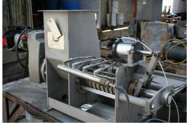
LAB PRESS STEAM INJECTION
