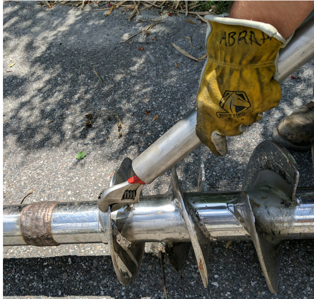
BENDING FLIGHT BACK INTO POSITION
