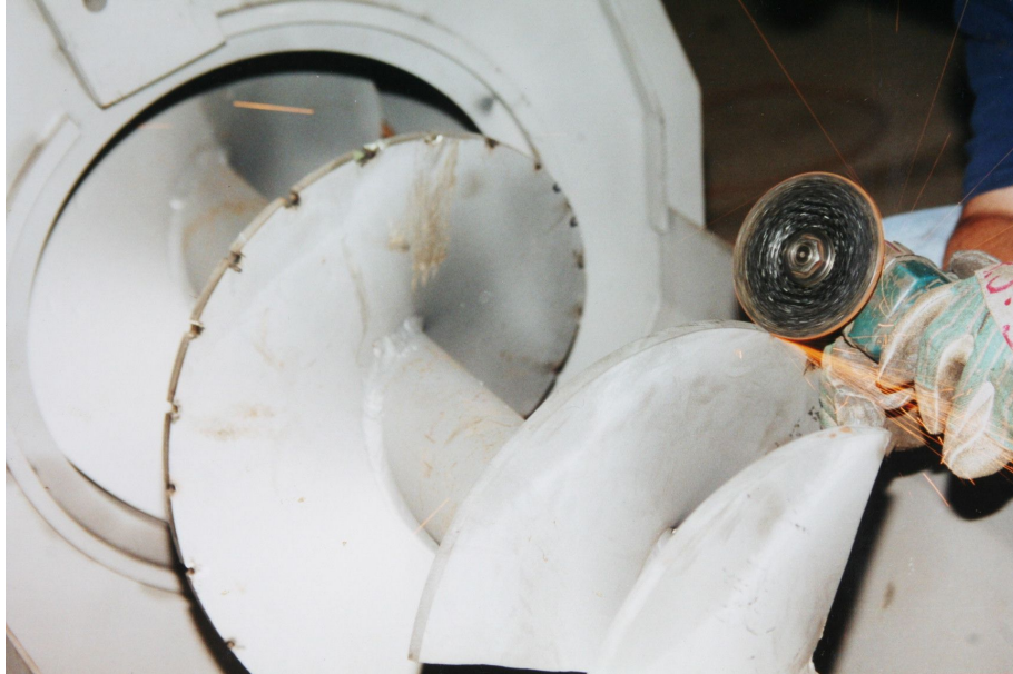
GRINDING NOTCHES IN THE FLIGHTS
