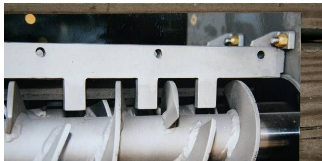
Interrupted Flight Screw with Resistor Bar
