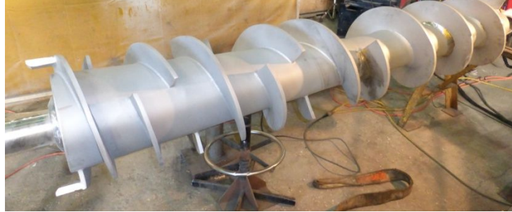
Screw with Tapered (Conical) Shaft
