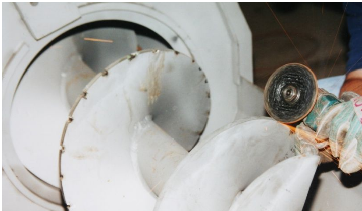
Grinding Notches on Screw Flights
