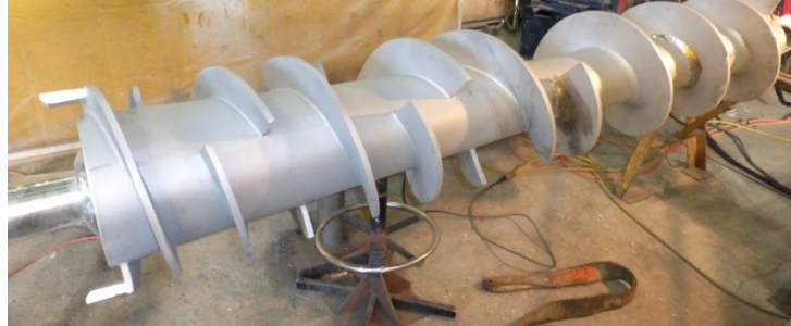
Screw with Tapered (Conical) Shaft
