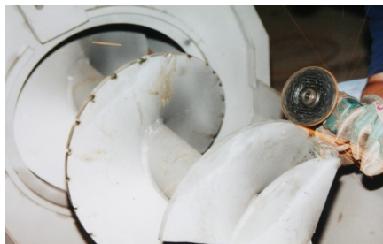
Grinding Notches on Screw Flights
