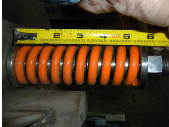
Spring Tightened to 5-3/8"
