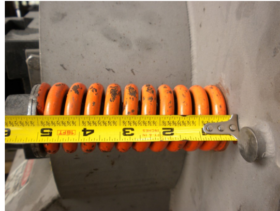
Spring Tightened to 5-1/16"
