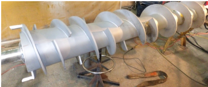
Screw with Tapered (Conical) Shaft
