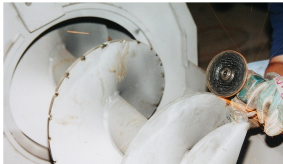
Grinding Notches on Screw Flights
