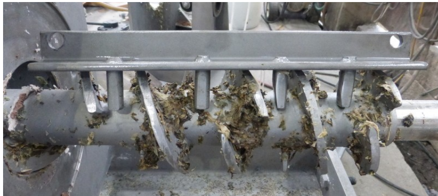
Interrupted Flight Screw with Resistor Bar
