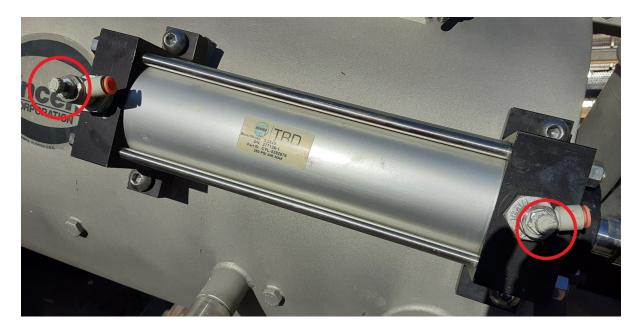
The backflush pump only sprays while the cylinder is moving *from* its resting position until the spray rings have traveled an entire stroke. The pump does not spray when the cylinder is returning *to* its resting position. The duration timer should be set to match the travel time of the full stroke from its resting position.
