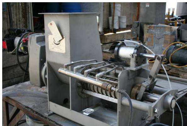
LAB PRESS STEAM INJECTION
