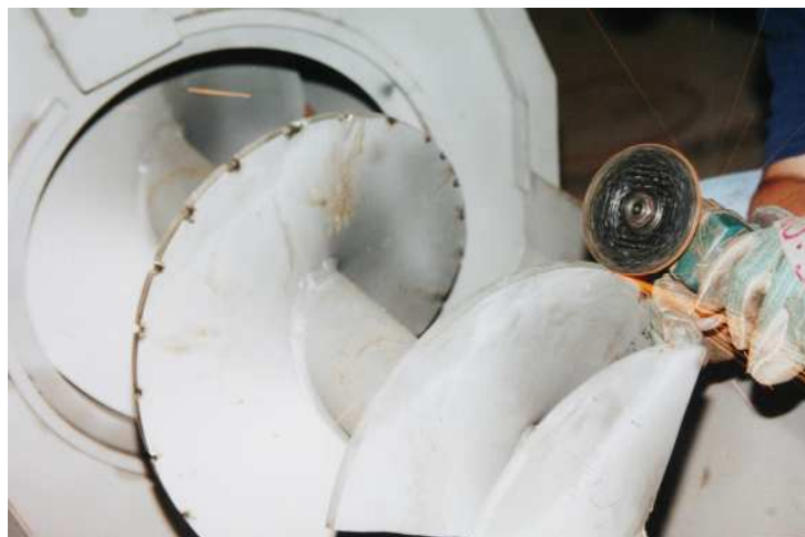
GRINDING NOTCHES IN THE FLIGHTS
