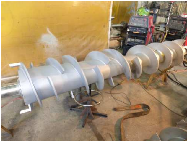
SCREW WITH TAPERED SHAFT (Note tightening pitch)
