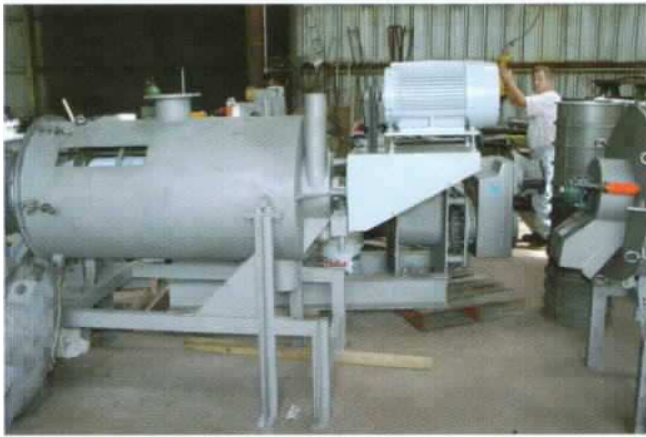
STEAM VENT ADDED TO FF-12 FOR HIGH TEMPERATURE APPLICATION
