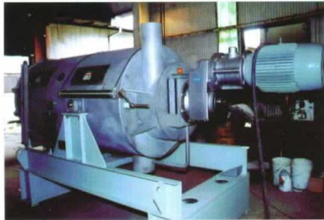
FF-30: ELEVATION IS ADJUSTED WITH AIR CYLINDERS SEEN IN THE BACKGROUND
