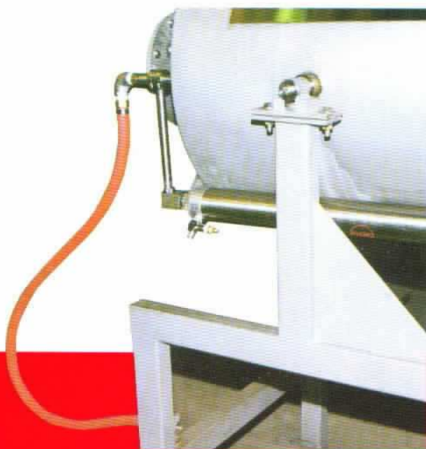
AIR CYLINDER ACTUATOR FOR BACKFLUSH SPRAY
