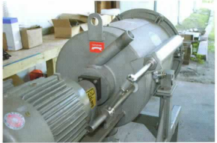
TANGENTIAL FLUID ENTRY ON FF-6
