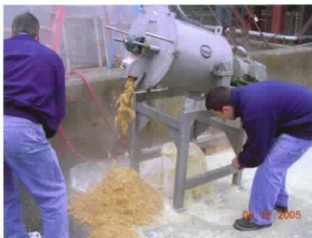
FF-6 FILTERING DISTILLERS SPENT GRAIN. NOTE THE DIRECT COUPLED ROTOR
