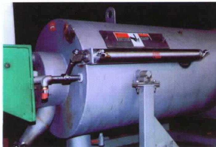
ABOVE AND BELOW: AN AIR CYLINDER ACTUATES THE TRAVELING SPRAY RING MECHANISM
