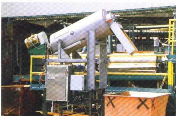
FF-12 FILTERING WASTEWATER AFTER DRUM SCREENS
