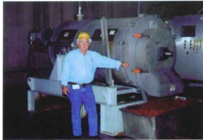
FF-30 FILTERING POTATO AND CARROT PEELER WASTEWATER
