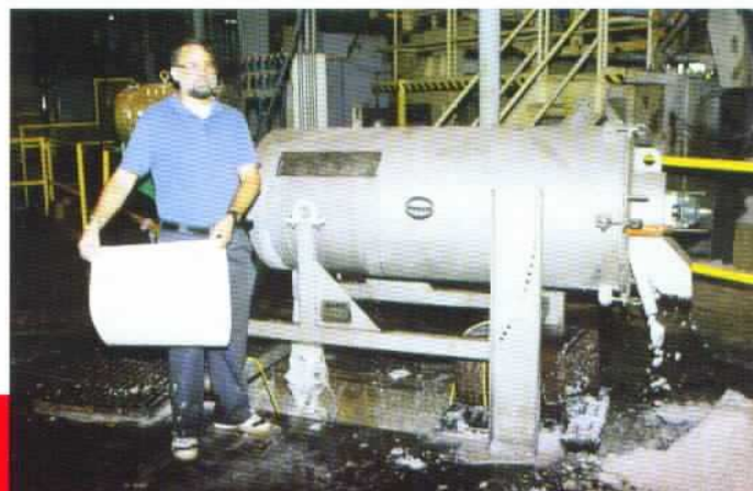
LOW SET ELEVATION FOR HEAVY CAKE DISCHARGE
