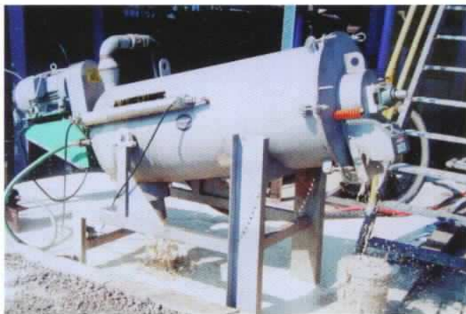
FF-12 SEPARATING FAT FROM BAIL WATER AT AN OIL FISH PLANT
