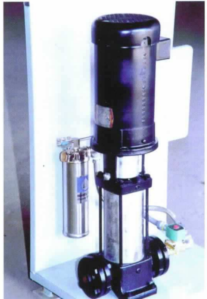
THE BACKFLUSH SYSTEM INCLUDES A FILTER, BOOSTER PUMP, SOLENOID VALVE AND CONTROL PANEL
