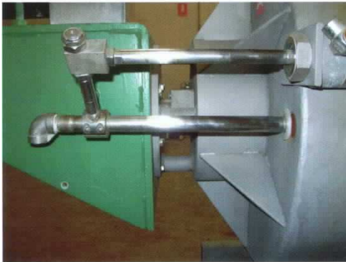
ABOVE AND BELOW: AN AIR CYLINDER ACTUATES THE TRAVELING SPRAY RING MECHANISM
