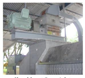
**Shredder at Press Inlet**
