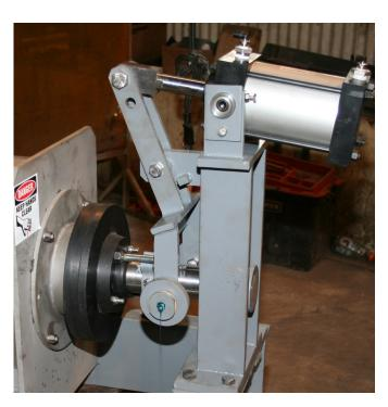
Air Cylinder Actuated Discharge Cone Controls Press Cake Moisture
